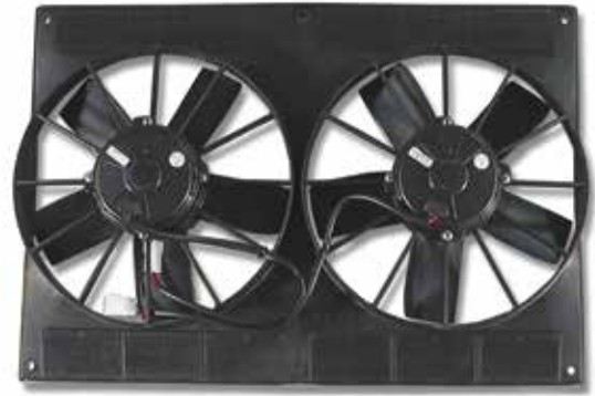
#58412 1990-1996 SPAL Dual 11" Fan Upgrade kit for DeWitt's 2-Row Core Radiators
